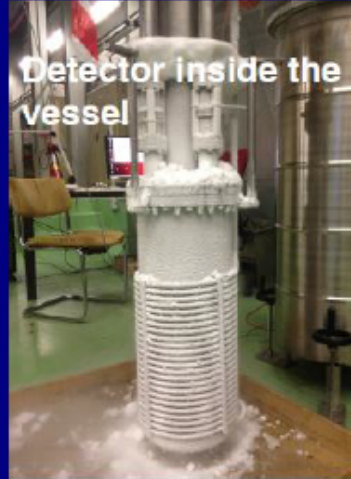
10x10x20 cm LEM-anode fast test setup
