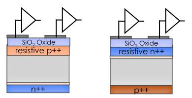
AC segmentation via resistive n++/p++ layer
