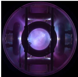
Figure: An EMC2 Polywell with a side length of 21.6 cm built for \beta=1 studies.
