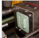
Detail of the core side in the injection machine
