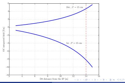
A simplified 2D model for tracking the BB effect for the D0
