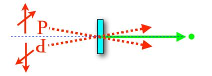
Two beams with image rotation: pointing instability is eliminated after frequency mixing
