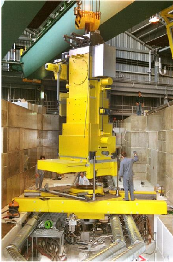
Exchange flask for meson production Target E (4 cm graphite wheel)
