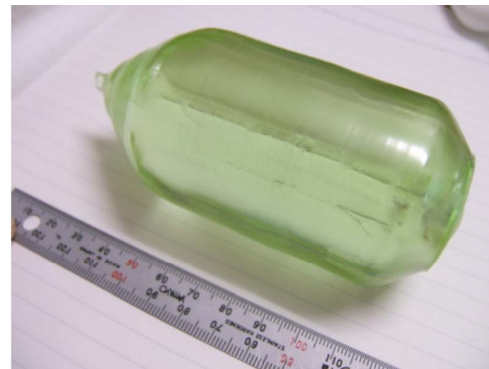
Crystal with Pr doping in 0.25 atomic%. 2in. diameter ingot
