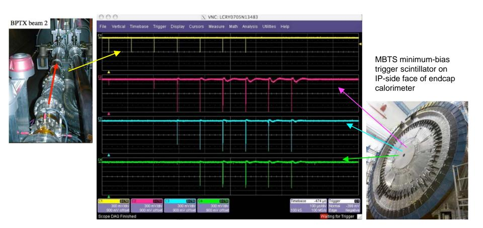
Beam losses evident for last few turns where BPTX trigger signal disappears but MBTS triggers appear and continue for two more turns (every  $89\mu s$ : single bunch, once per orbit)
