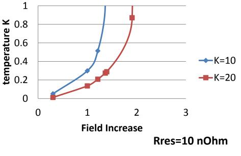
If the Nb has a low RRR (k=10) AND is dirty ( $R_{res}=10$ ) then we may have an issue. Otherwise it is capable of 5 MV operation.
