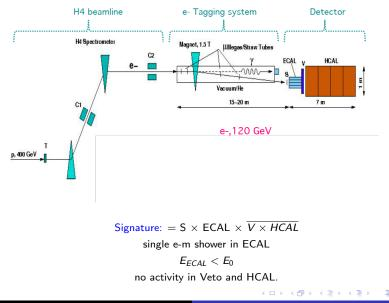
$\rightarrow$  Detector tests and calibration with  $e^-,$  pion, kaon and proton beams.
