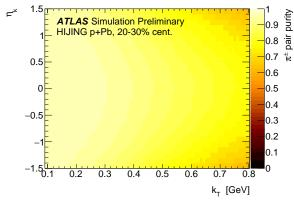
The pair purity for the nominal selection, estimated from simulation, is shown above as a function of pair  $k_{\rm T}$  and  $\eta_k$ .
