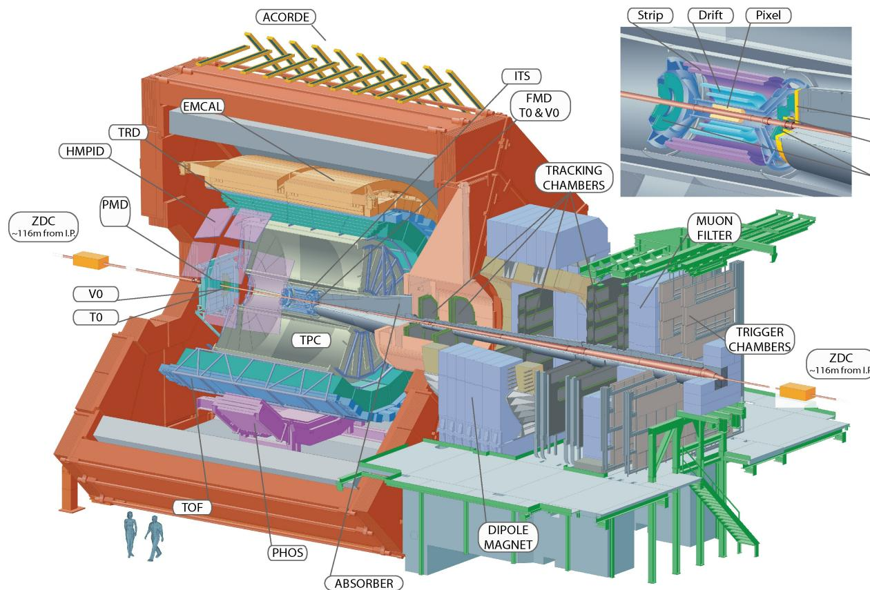
Sub-detectors used for measurements of  $dN_{ch}/d\eta$ :
