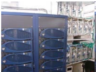
Gescher Cluster (80 processors), a subcluster of single CPU nodes, a subcluster of 4xCPU SMP nodes
