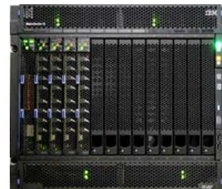
Celline, 1xLS22 & 4xQS22 (2xQuadCoreOpteron & 8xPowerXCell8i)
