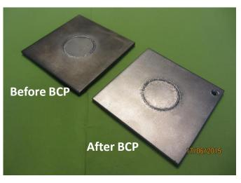
Flat welding trials: needed for setting weld parameters
