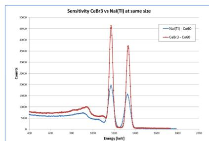
Figure 2: Comparison of Co-60 spectra for  $\text{CeBr}_3$  (red) and  $\text{NaI}(\text{Tl})$  (blue), each 2"x2" in size.
