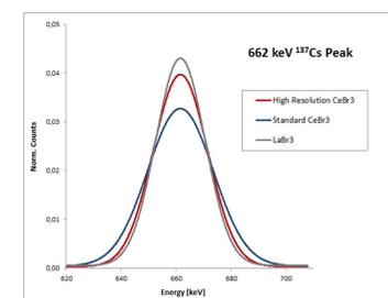
Figure 7: Improvement in energy resolution of  $\text{CeBr}_3$ . 1"x1"  $\text{CeBr}_3$  crystal with 3.5% resolution at 662 keV (red) in comparison with Standard  $\text{CeBr}_3$  (blue) and  $\text{LaBr}_3$  (grey).
