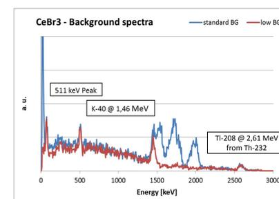
Figure 5: Improvement in intrinsic activity of  $\text{CeBr}_3$ . Low Background  $\text{CeBr}_3$  (red) in comparison with Standard BG  $\text{CeBr}_3$  (blue). Most of the peaks in the (red) Low BG curve are unrelated to crystal activity, stemming from cosmic radiation (511 keV peak) or environmental sources (K-40 and Th-232).
