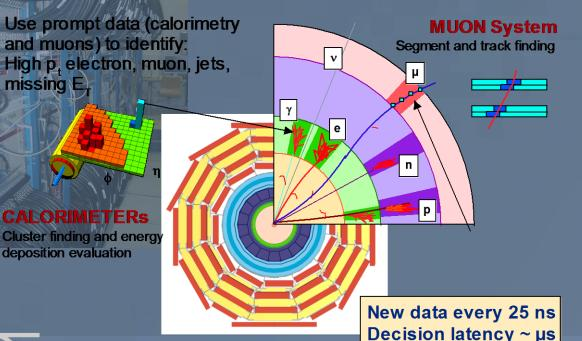
A combination of (radiation hard) ASICs and FPGAs process data of "simple" sub-systems with "few" O(10000) channels in rèal-timé
