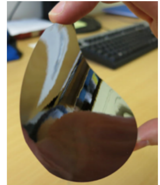
50 \mu\text{m} thick silicon wafer
