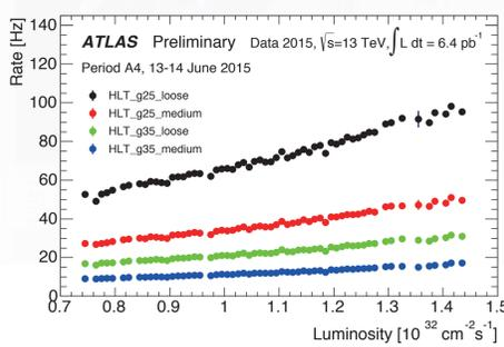
Output rates of single electron triggers as a function of the instantaneous luminosity. Medium-quality identification criteria will move to tight selections for higher luminosities.
