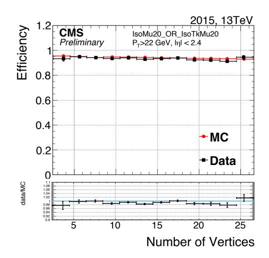
efficiency of the **OR of HLT\_IsoMu20 and HLT\_IsoTkMu20** on the top of offline muon identification and isolation in the 50 ns LHC data
