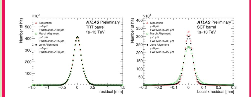
Changes in the environmental conditions may lead to movements of the ID. June 2015 collision data have been used to study the stability of the detector between runs.
