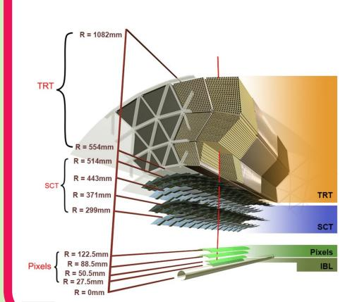
During the Long Shutdown 1 (LS1) several manteinance works were performed together with the installation of new detectors. Alignment has thus become a major task during the cosmic campaign and first 13TeV collisions in order to get the detector ready for the stable beams. An important part of the ID alignment has been the study of the IBL performance. The IBL is a new pixel layer attached to the beam pipe which had never been aligned before.
