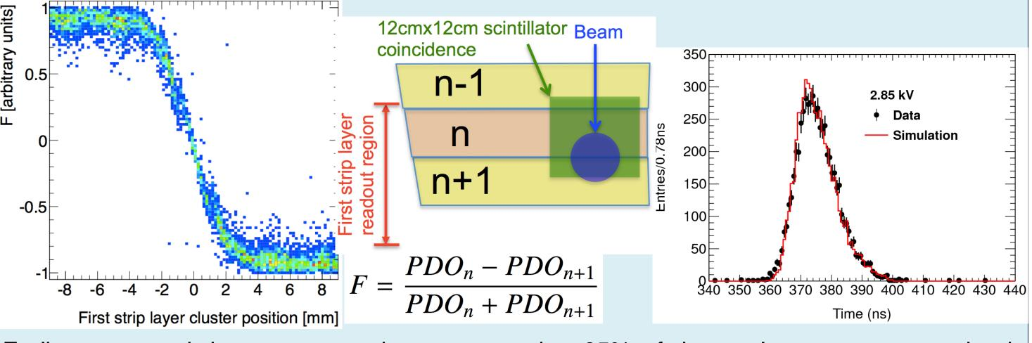
Earlier measured time spectrum demonstrates that 95% of the total events are contained within a 25 ns time window.
