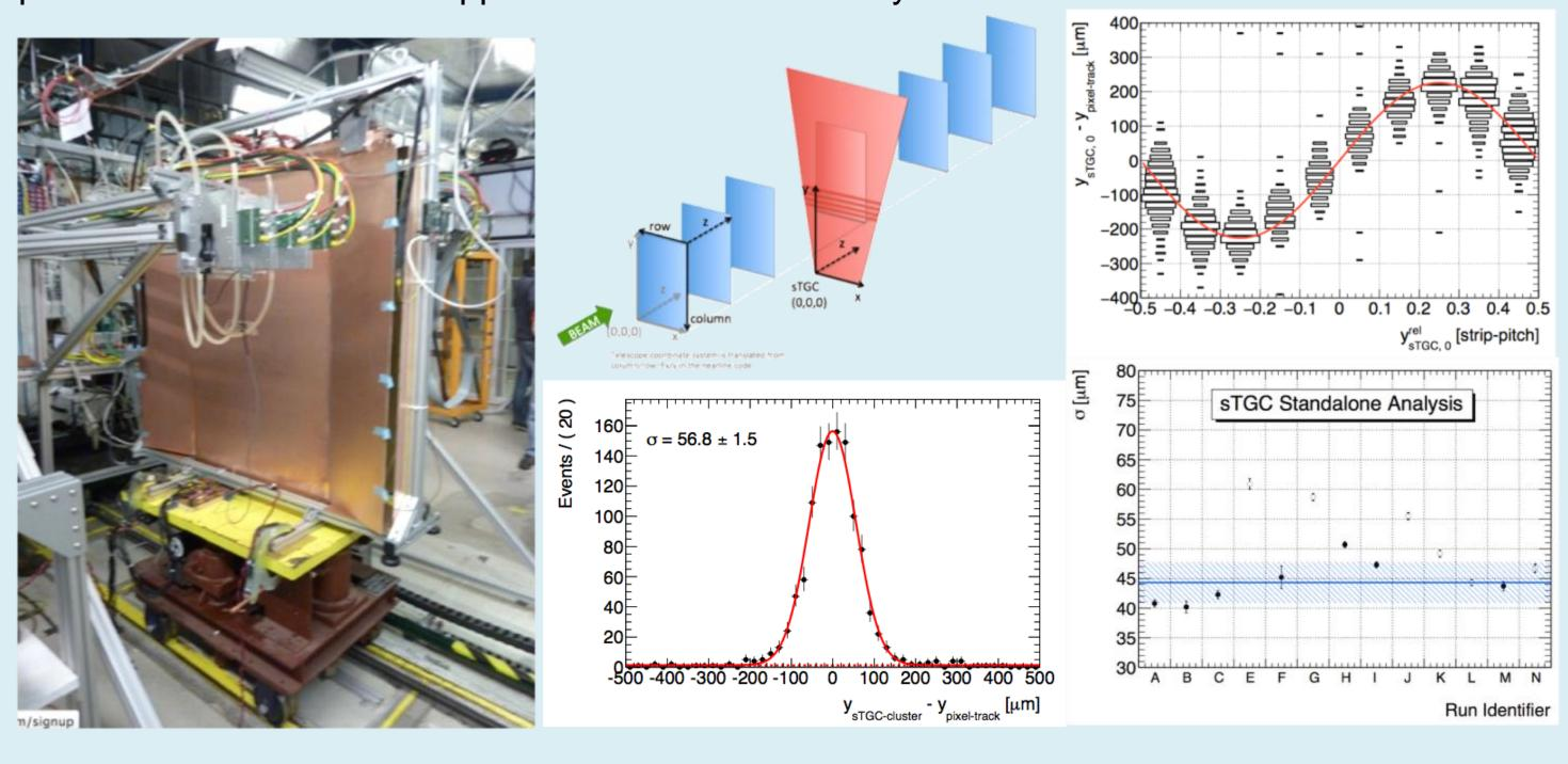
At the CERN test beam, the charge sharing between pads was measured by centering the beam (130 GeV muons) in the transition region between two pads. The charge fraction (F) is defined using the analog peak values (P) of two neighboring pads. The transition region, defined as |F| <0.7, is measured to be about 4 mm.
