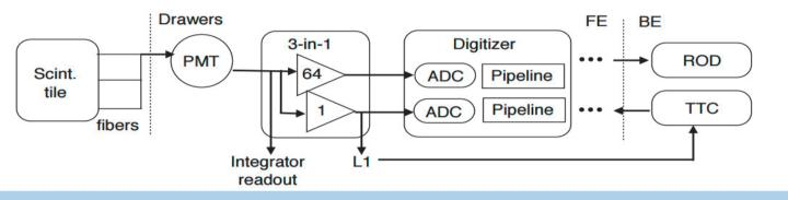
■ The signal from the PMTs is shaped and amplified using two gains (1:64) with 10-bits ADCs each 25 ns
