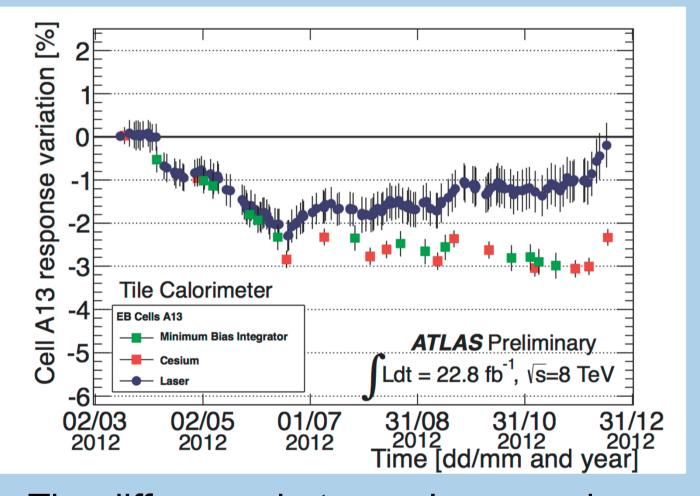
■ The difference between Laser and Minimum Bias (or Cesium) response gives the effect of the scintillators irradiation (~ -2% max in 2012)
