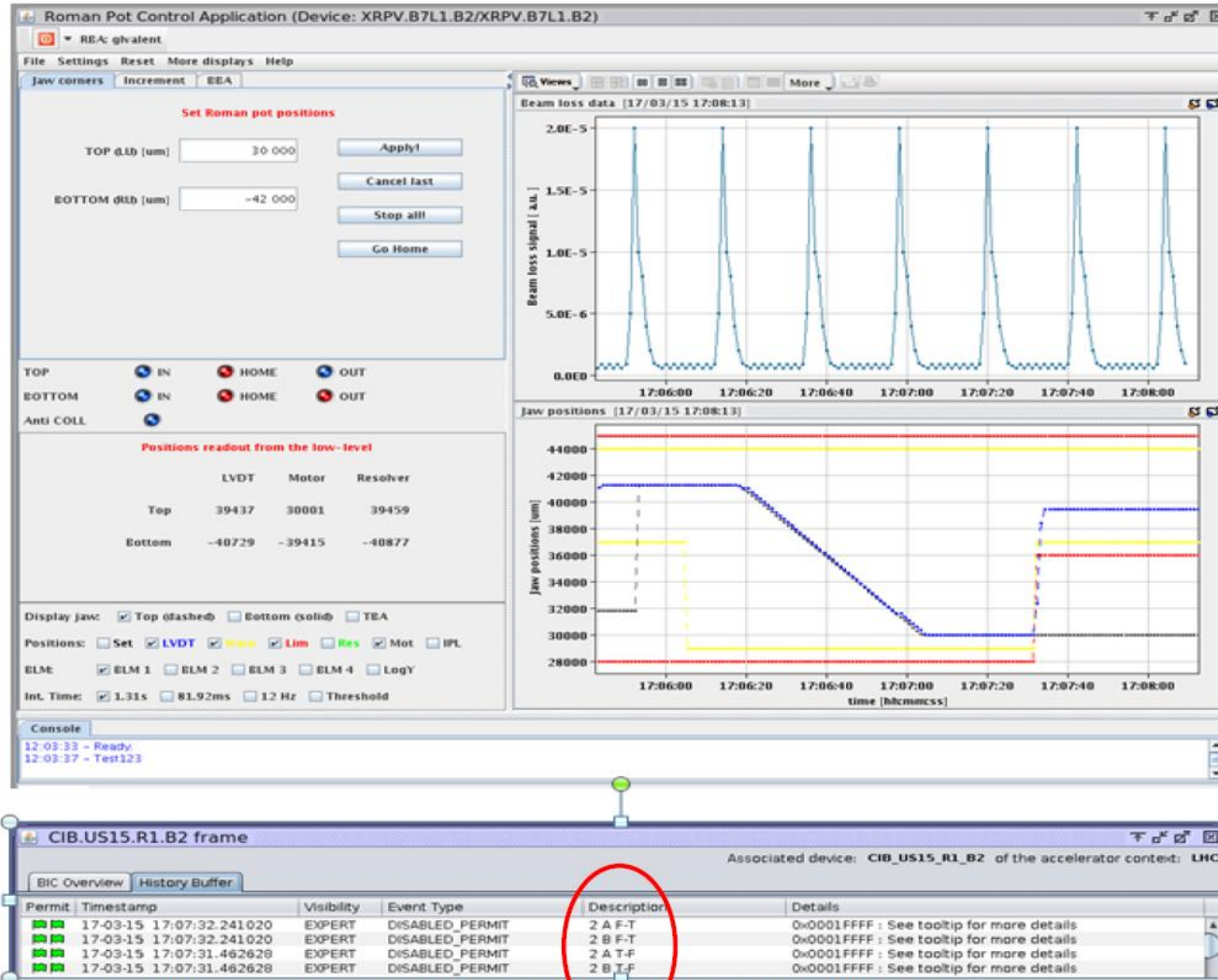
Figure 4. TOP : Collimator application used to move Roman Pot B7L1 Upper. BOTTOM : Corresponding loss of INJECTION_PERMIT seen in the BIS history buffer.
