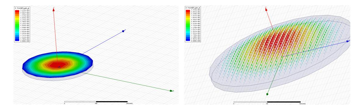
E-field as a function of distance from the center of the cylinder
