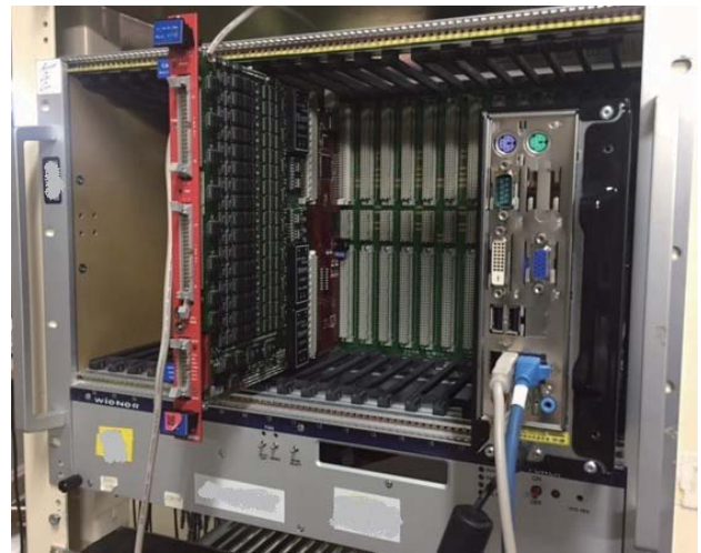
Fig. 3. Photograph of the installation in the VME crate. MOCO is inserted between the VME module and the VME bus.
