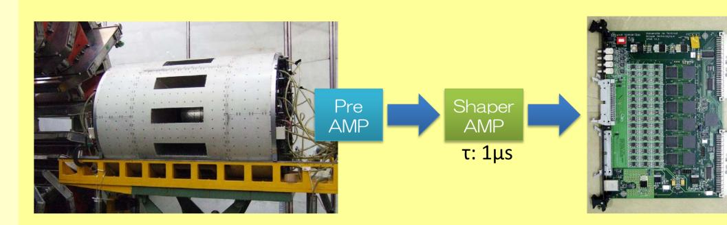
TRIUMF VF48 waveform sampler
