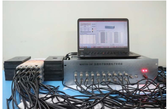
Fig. 1. Photo of the readout system which has 20 neutron detectors (crystal ST-401 and PMT), the electronics system and the software.
