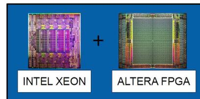
Fig. 1. Intel Xeon/FPGA prototype used for the tests. This is two socket server machine, one with Xeon CPU and the other with Altera FPGA.
