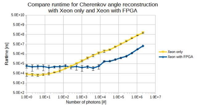
Fig. 2. Time for reconstructing the Cherenkov angle on a CPU compared to the runtime on an FPGA.
