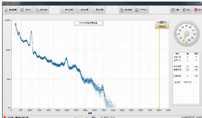
Fig.6 The energy spectrum acquired by PGNAA DAQ
