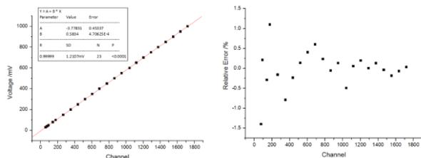
Fig.4 The linearity (left) and the relative error (right) test of the readout system.
