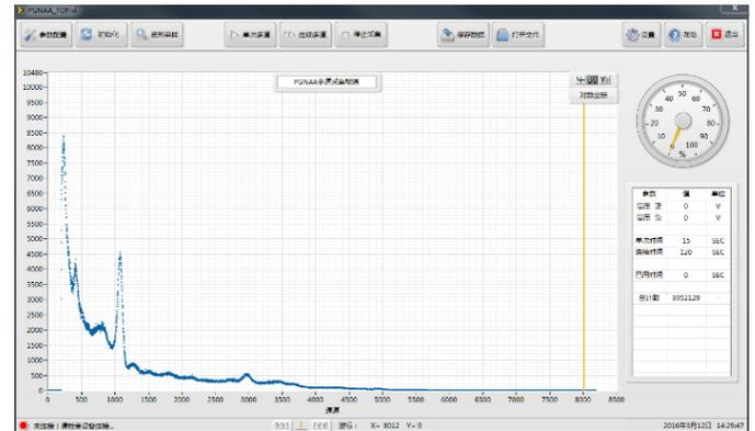
Fig.2 The photo of the GUI pane. This panel can help setting the threshold of the peek-seeking module, the control voltage of the high voltage control module, and the parameters of sequential control. And it also provides a function of energy spectrum display and analysis
