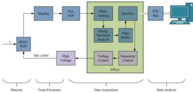
Fig.1 Block Diagram of PGNAA Readout System
