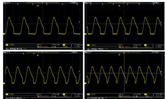
Fig.3 The signal outputted by the shaping circuit, upper-left 5MHz, upper-right 6MHz, lower-left 7MHz, lower-right 8MHz.
