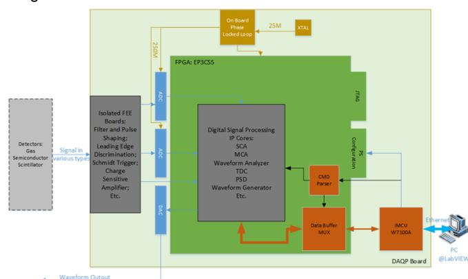
Fig.2. Schematic Block diagram of the DAQP System
