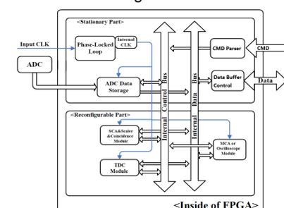
Fig. 4. FPGA internal logic block diagram
