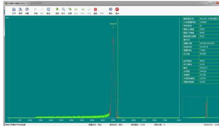
Fig. 6 Alpha energy spectrum of <sup>241</sup>Am
