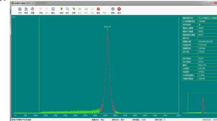
Fig. 7 Alpha energy spectrum of <sup>239</sup>Pu
