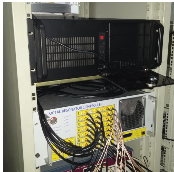
Fig. 3. Rack. On the top there is the PC and under it there is the OCR
