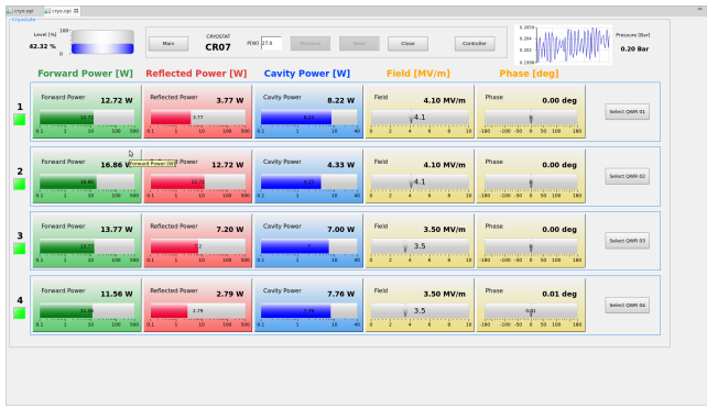
Fig. 4. CSS Interface for monitoring the working status of a cryostat. In the top corners the level of liquid Helium in the cryostat, on the left, and the pressure of the Helium, on the right, are monitored. For each cavity there is the possibility to read the forward power, the reflected power, the power in cavity, the gradient of the electric field and its phase in cavity.
