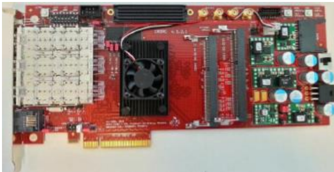
Fig. 1. C-RORC hardware: on the left the optical transceivers, in the center the FPGA, under the fan, and the PCIe interface.
