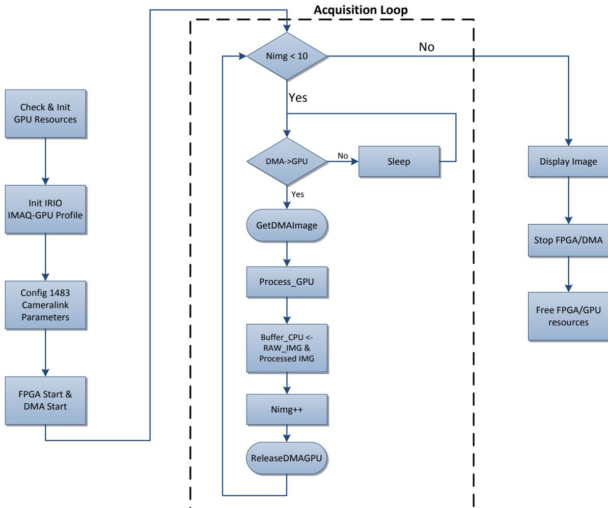
Figure 2: Flowchart of FlexRIO\_mod1483-7966-Imag-GPU.c
