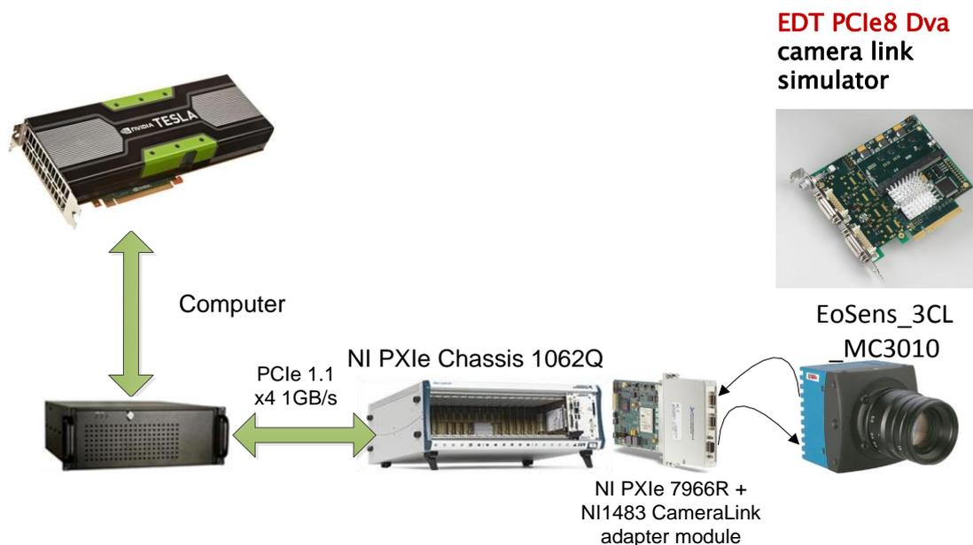
Figure 1: Architecture of the image and processing system implemented with PXIe Technology
