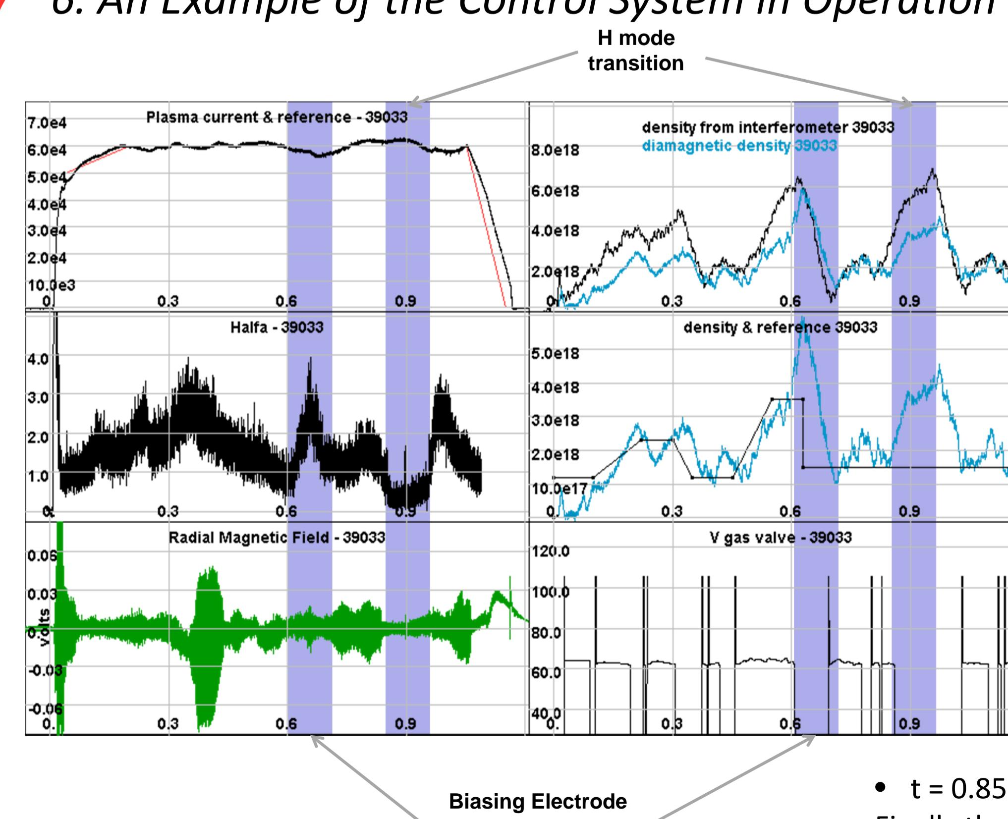
An experiments with a biasing electrode applied to the plasma
