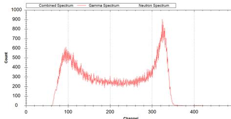
Fig. 5. The multi-channel analyzer (MCA) graphical-interface with unfiltered gamma-only pulse-height spectrum of data acquired from an EJ309 liquid scintillator positioned 45 mm from a Cs-137 source.
