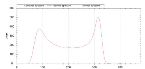
Fig. 6. The multi-channel analyzer (MCA) graphical-interface with 20-point moving-average filtered gamma-only pulse-height spectrum of data acquired from an EJ309 liquid scintillator positioned 45 mm from a Cs-137 source.
