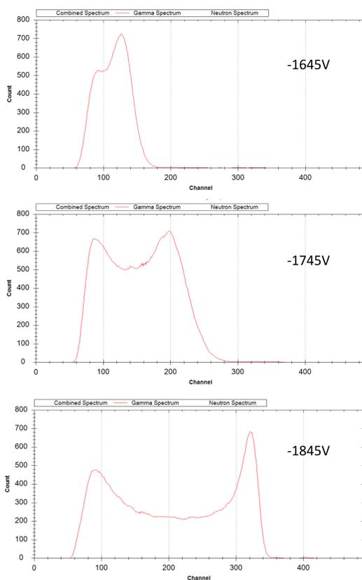
Fig. 2. Cs-137 spectrum with 10-point FIR filter acquired from an EJ309 liquid scintillator operated with a negative bias of 1645, 1745 and 1845 V in descending order. The photon peak locations are at channel 130, 200, and 320, respectively, on the MCA.
