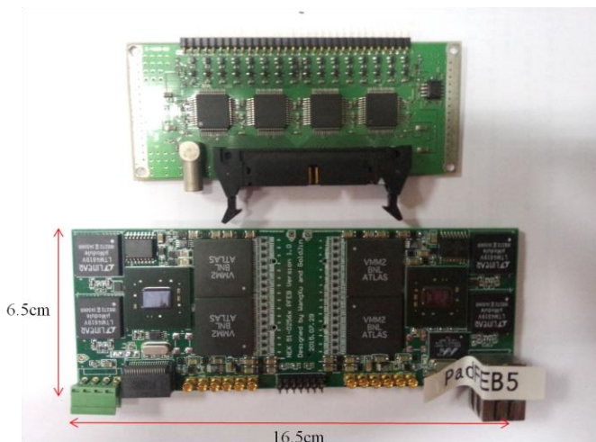
Fig. 2. The photo of the pFEB(bottom) and the former FEB(top).
