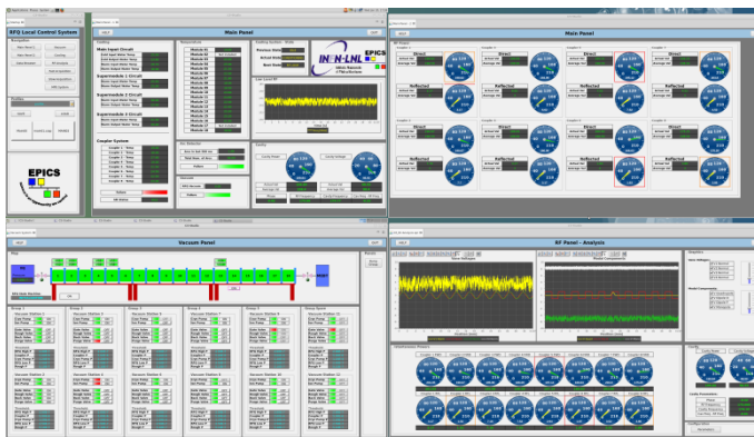
Fig. 3. GUI developed for the RFQ local control system.
