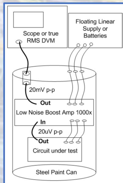
Figure 2: noise measurement setup
