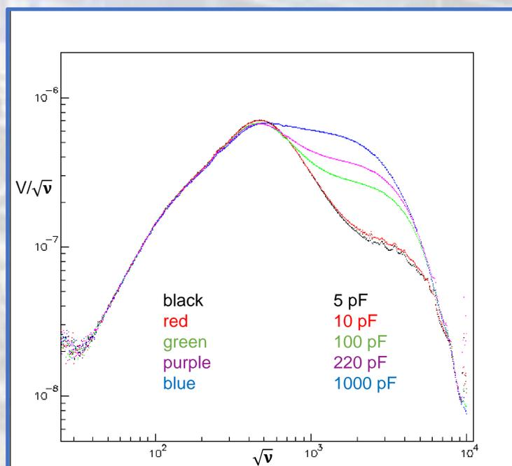
Figure 4a: the pre-amp has been loaded with different capacitance
