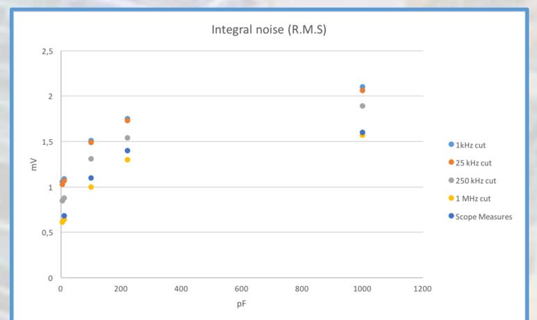
Figure 4b: integrated noise spectra compared to the noise measured by the scope.
