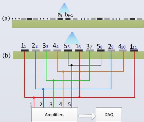
Fig. 1. Principle of encoded multiplexing method
