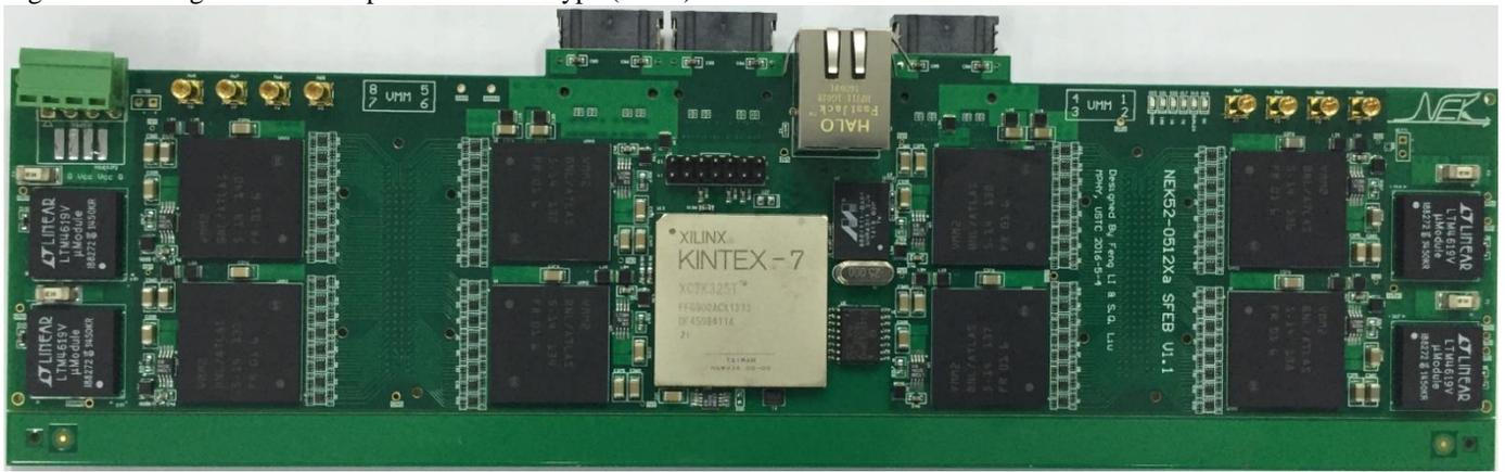
Fig. 2 the photo of sFEB(top view, Mini-SAS connectors are on the bottom layer, the RJ-45 connector will be replaced with another Mini-SAS in the final version)
