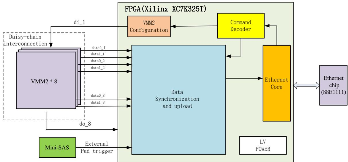
Fig. 1 Block diagram of the strip Readout Prototype (sFEB)
