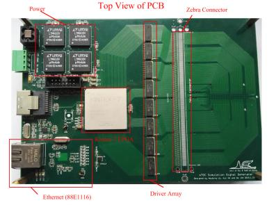
■The GEM prototype has been applied in pFEB (pad frond end board) and SG (signal generator). The Ethernet interface is response for the communication between pFEB and PC or SG and PC.
