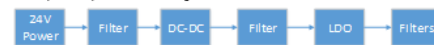
Figure 3 Block diagram of the power generating and filters of the power system
