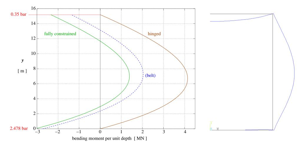
"belt": heavy beam 1200 / 550 / 40 / 75 [mm] all around; including own weight; deflections x 150; max. deflection = 19 mm
