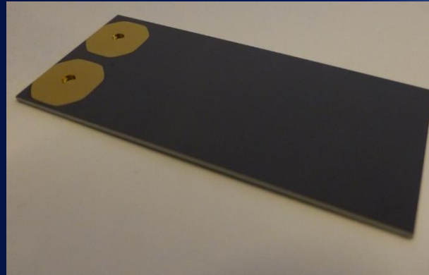
Soldering test with metallized ceramic on silicon
