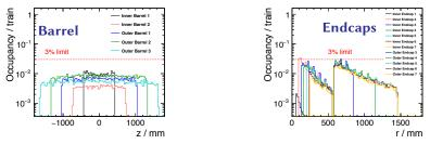
• Readout granularity defined by the backgrounds occupancy of  $\sim 3\%$   $\Rightarrow 50\,\mu m$  pitch and 1-10 mm strip lengths.
