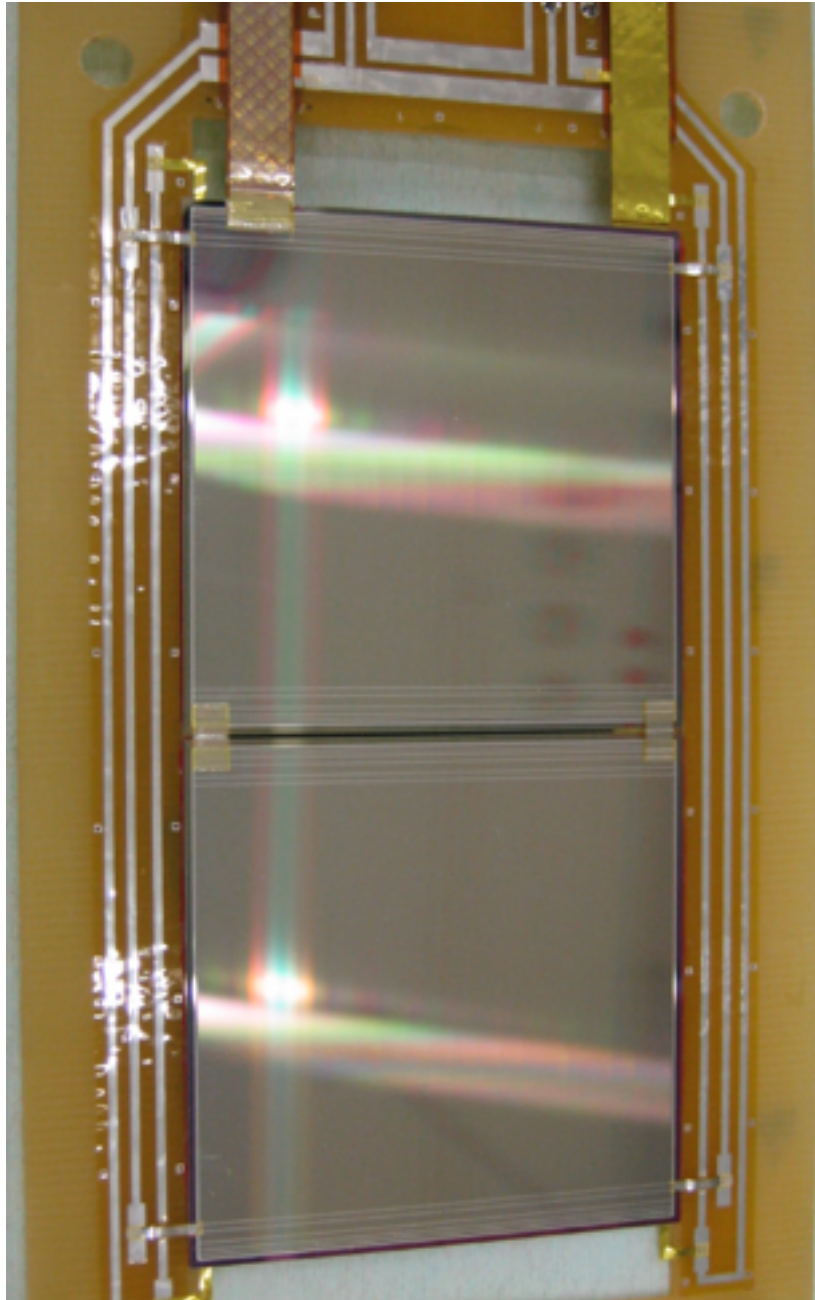
two daisy-chained sensors
