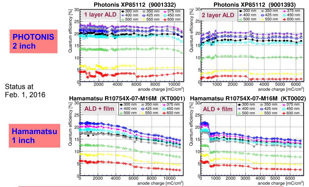
Albert L All ALD coated MCP-PMTs with >5 C/cm<sup>2</sup> integrated anode charge !
