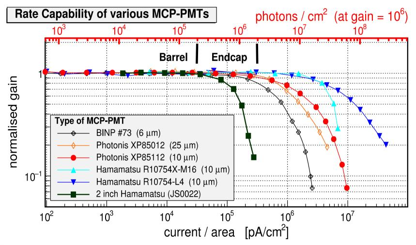
most MCP-PMTs show stable operation to ~200-300 kHz/cm<sup>2</sup> single photons (at gain 10<sup>6</sup>)
