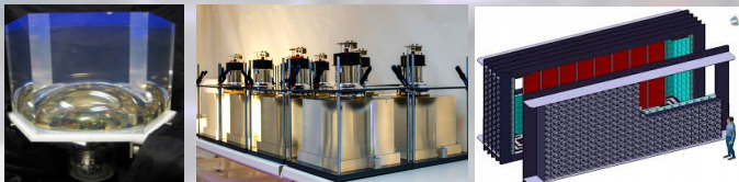
Fig. 4. Scintillator blocks (256 mm x 256 mm 2 ) made from Evninet polystyrene plastic scintillator are directly coupled to 8" photomultiplier tubes (R5912-MOD Hamamatsu).
