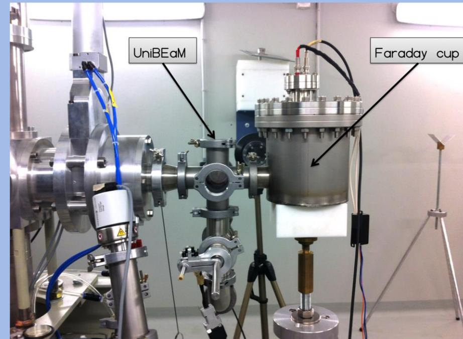
Beam tests with a continuous
